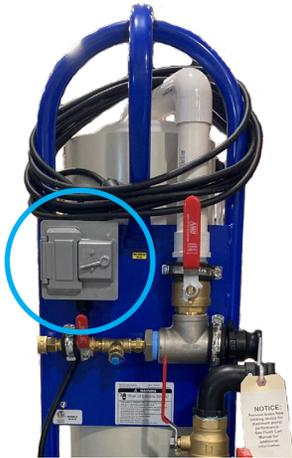
**Figure 21: Remove electrical box from cart.**
