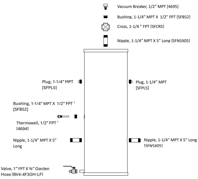
1. HCT-R2 20 Gallon buffer tank does not have a thermowell port.
