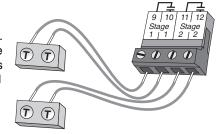
Sensor and Unpowered Input Connections
